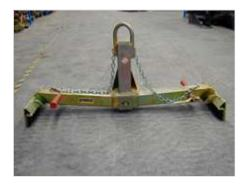
Especially suitable for handling concrete kerb stones and paving slabs. The one-sided angular supports which are placed on the kerb stone, already in place to enable an extremely narrow joint.
